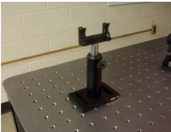
**Figure 10:** This figure shows the custom-made microscope slide holder constructed to mount on our existing optics posts.
